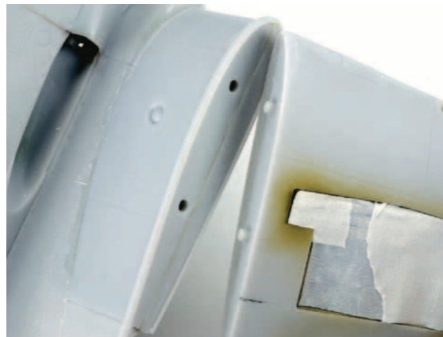
Location for the outer wing section is taken care of with the pegs but they need a little trimming to get them to fit inside the raised reinforcing rib. Once in position it makes for a very sturdy joint
