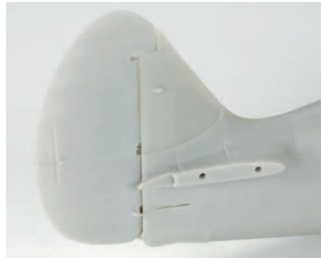
At the other end of things we have the tail, with additional control rods made from stretched sprue and the tip of the fin made into the proper shape with more talc n'glue. Note the welcome addition of locating pegs for the horizontal stabilizers
