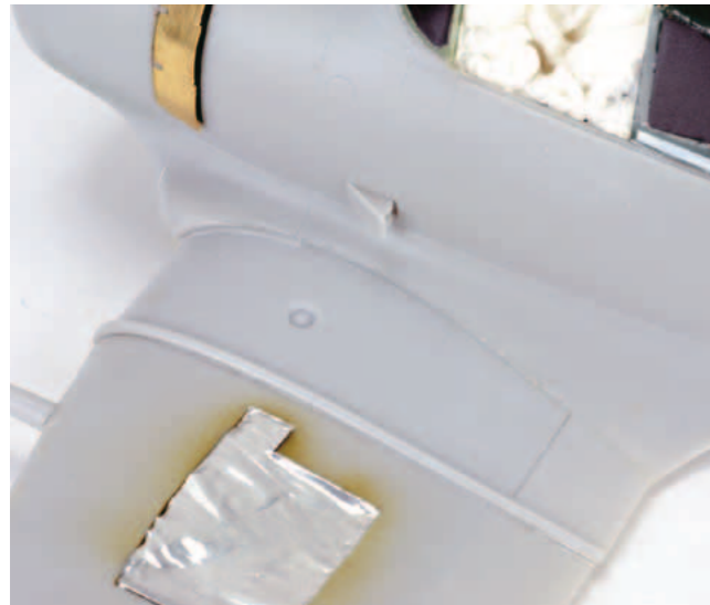
The wing root joint is as good as it gets in this medium, showing that Alley Cat have taken some care over the casting processes
