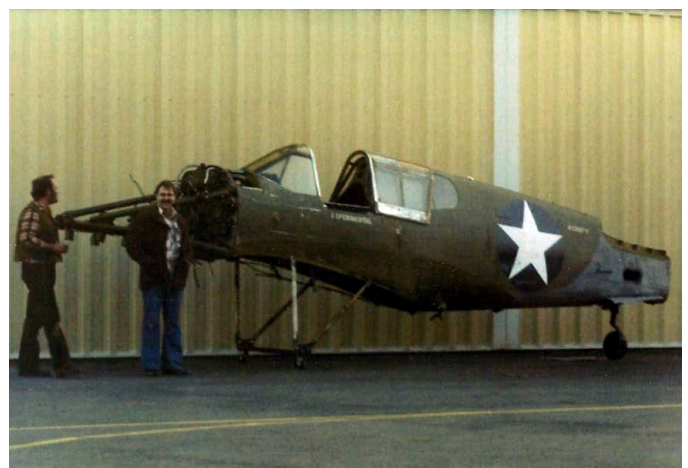
▲ With a temporary steel dolly replacing its main landing gear, the P-40’s fuselage could easily be rolled around like a big toy.
