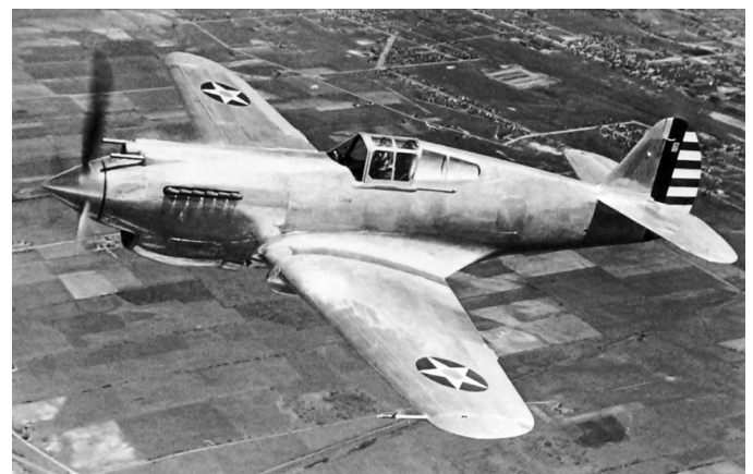
▲ The XP-40 was the 10 th production P-36A Hawk airframe fitted with a liquid-cooled, supercharged Allison V-1710 V-12 engine in place of its original air-cooled Twin Wasp radial.
