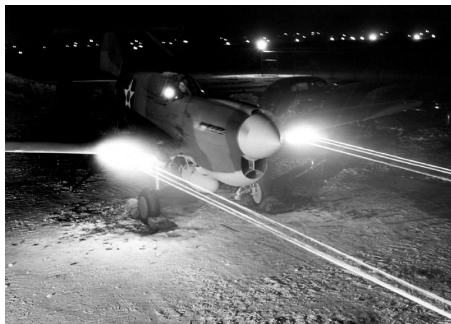
▲ Starting with the P-40D, the Warhawk's armament was six hard-hitting .50-calibre Browning machine guns, three in each wing. Deadly to the enemy, it also made for an impressive display on the firing line as the guns were harmonized, i.e., set so that their streams of fire converged at a certain range.
