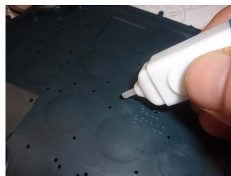
CA application into the keyed bezel from the backside of the panel will suffice in fixing the item in place. This will also aid in avoiding messing up the painted components that could occur if the gluing process was made at the front of the panel, and also the damage that the fumes of the CA could cause on the clear parts.
