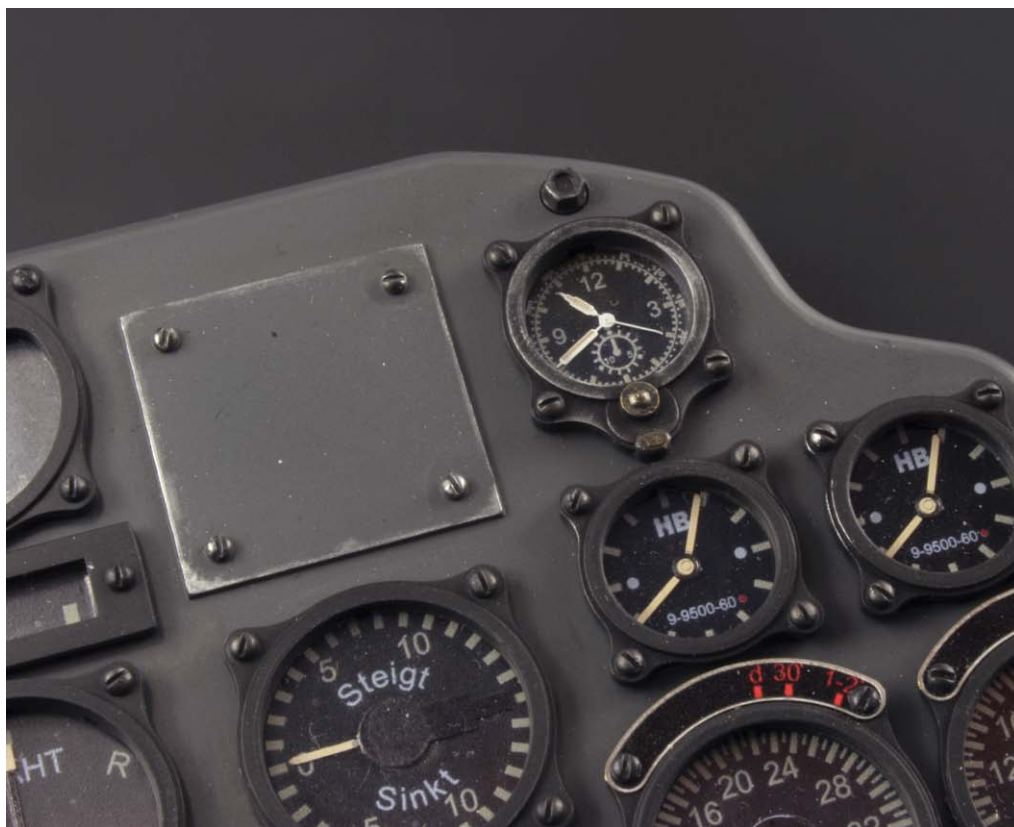
Upper right portion of the panel with the clock and patch over an unused instrument space.
