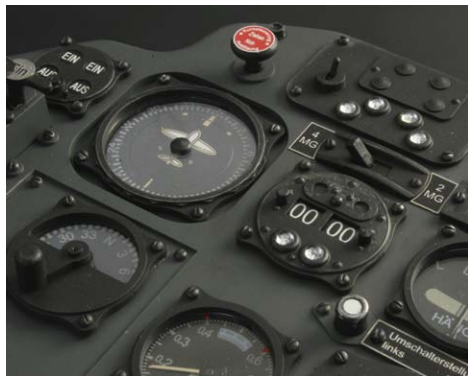
The final look of the middle section of the panel, with painted instruments and limit indicators on the altimeter and air speed indicator.
